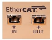
The input, labeled "IN" is used to control the BX18 over EtherCAT. The output is labeled "OUT" and is used optionally if the application requires multiple EtherCAT devices on the same bus and the arc generator is not the last device on the daisy chain.
